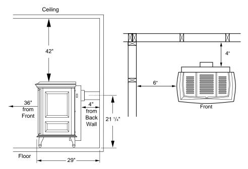
Figure 3 - Clearances for Standard Installation
